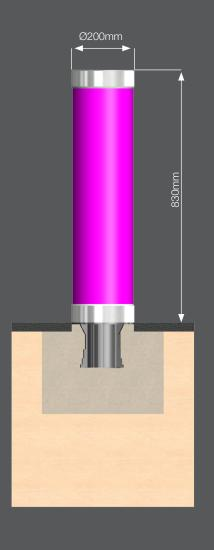
Supplied with dedicated embedding base which make installation/removal easy using a flat wrench 13 only. Maintenance requires a socket wrench 10, an Allen wrench 5 and a plastic hammer.
